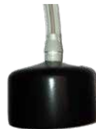
Calibration Cup Assy, IR-RS Cup Inner Diameter: 42.8mm Tubing Inner Diameter: 5mm Note: The cup has four equal cuts to allow it to fit over the IR-RS sensor as shown below. Usage: IP41 units with IR-RS sensor
